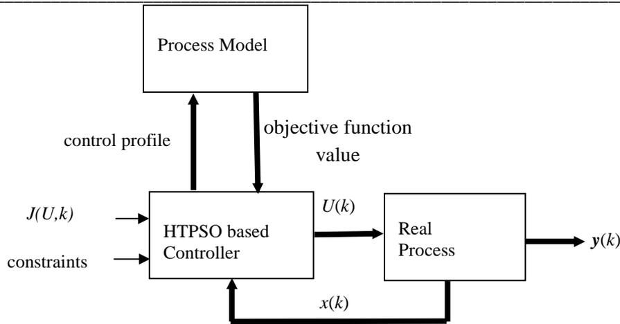
Fig. 3. Control Structure with PSO based Controller
