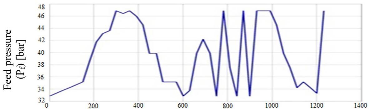
Fig. 7. Time pressure fluctuations within the desalination plant [19]
