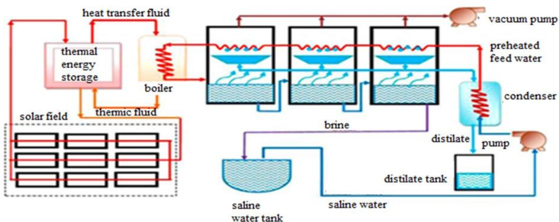
Fig. 1. Experimental installation of desalination using solar energy [14]
