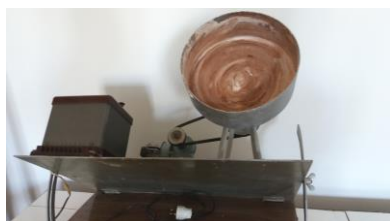
Fig. 4. Laboratory installation for pelletization
