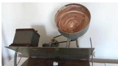
**Fig. 4.** Laboratory installation for pelletization
