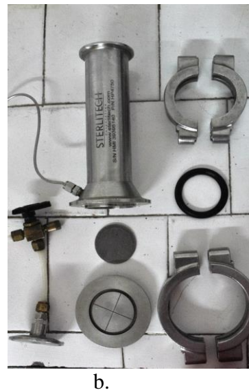
Fig. 2. Dead-End Filtration System: a. filtration plant; b. filtration cell
