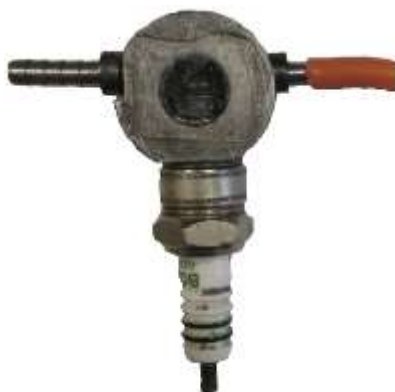
Figura 3.7. Reactor de plasmă Gliding-Spark (Nox Box)
