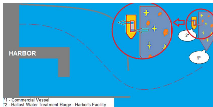
Figure 5.9 Port facility - ballast water treatment barge [32]
