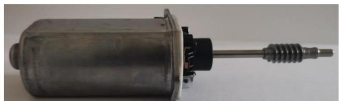
Fig. 5.9. The worm shaft from the construction of the seat adjustment mechanism of a Mercedes car
