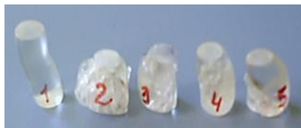
Fig. 5.1. Stress/strain curves for the studied resins and images of the tested specimens (compression)
