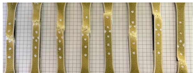
Fig. 16 \sigma/\epsilon curves and tested specimens for CM materials
