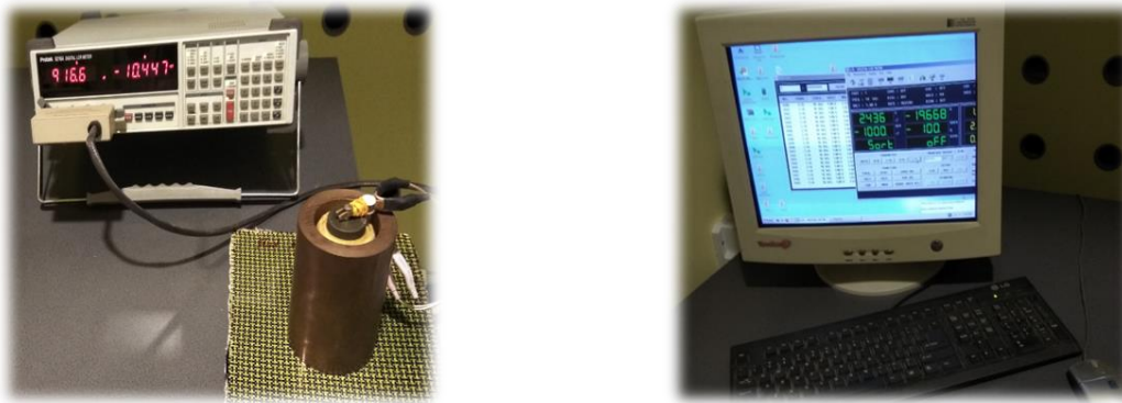
Fig. 3.12. Protek RLC meter and measuring cell. Application interface made at CCDCOMT
