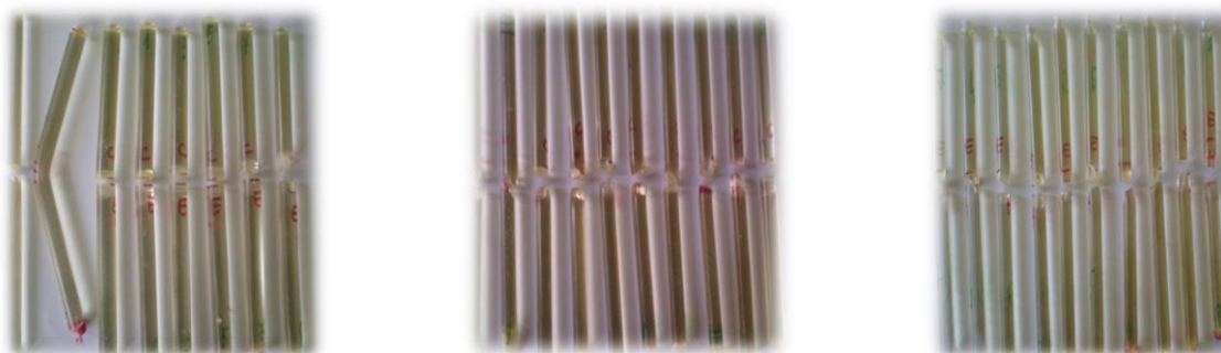
Fig. 6.3. Specimens tested in three-point bending (materials containing junctions – CE, CH, EH)
