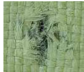
Figure 5.40. Detail of layer 1 (Twaron SRM509 fabric), Fire A, of the 32-layer hybrid panel, back view
