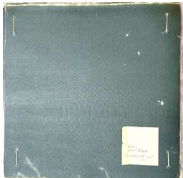
Figure 4.8. How to fasten the Twaron SRM509+ Twaron CT736 combined fabric layers panel
