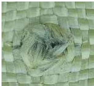
Figure 5.35. Detail of layer 1 (Twaron CT736 fabric), Fire A, of the 16-layer Twaron CT736 fabric panel, front view
