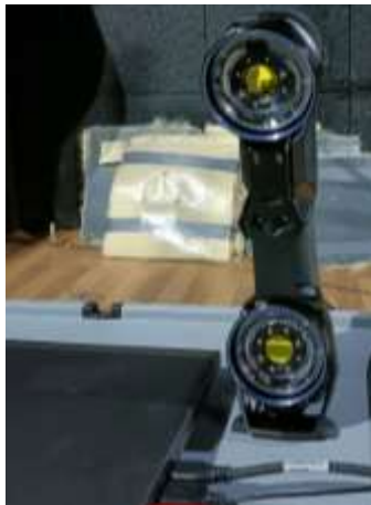
Figure 5.2. Measurements HandyScan 3D scanner
