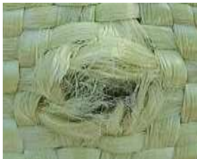
Figure 5.39. Detail of layer 1 (Twaron CT fabric), Fire A, of the 32-layer Twaron CT736 fabric panel, back view
