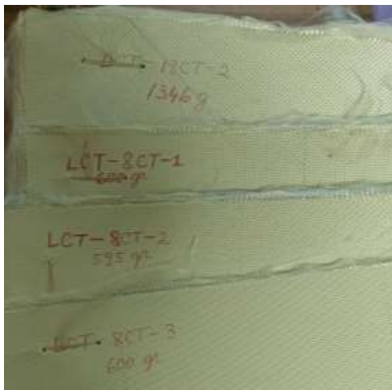
a) Sewn panels forming the 42-layer Twaron CT736 fabric panel
