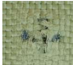
Figure 5.36. Detail of layer 1 (Twaron SRM509), Fire A, of the 16-layer combined Twaron SRM509 panel, back view
