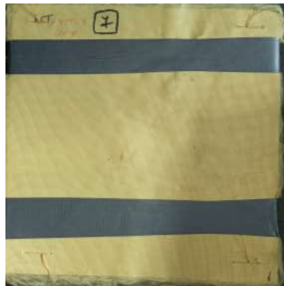
b) 42-layer panel fastened with textile shells
