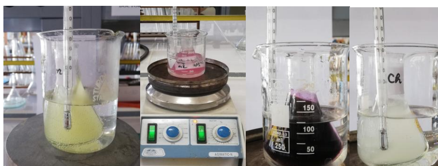
Figure 4.9. Images of synthesis process for the chitosan derivative CHS
