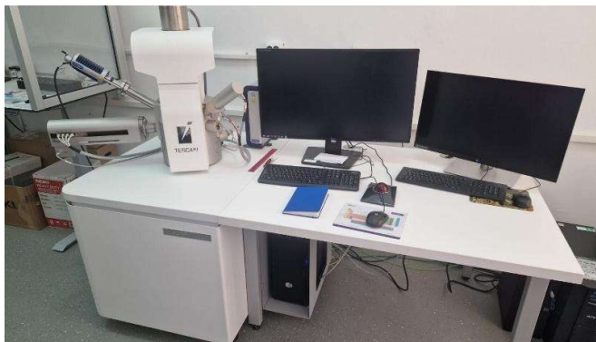
Figure 3.2 of SEM TESCAN VEGA equipment (photo Georgiana Ghisman)
