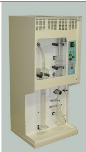
Figura 4.3. Distilator automat ENODEST
