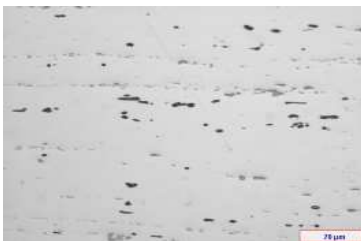
Fig.4.8. M=200X Cod TT 4.1/ t= 13h/ T = 165°C M=200X Atac 0,5% HF
