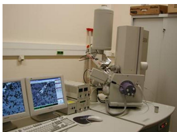
Fig. 2.20. Microscopul electronic cu scanare, Philips XL 30 FEG
