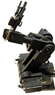
Fig. 3.8 Manipulator robotic Pioneer 5-DOF
