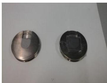
Figure 2.18 Sample support for XRD analysis
