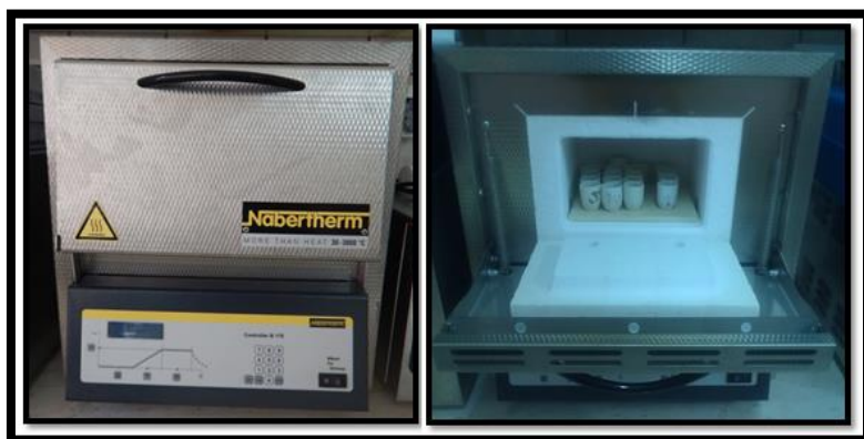
Fig. 2.33. Cuptor de calcinare tip Nabertherm (foto original)
