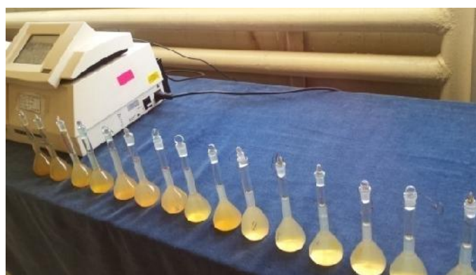
Fig.5.2. Volumetric flasks with sonic/ultrasonic treated water samples, during the determination of the ammonia content by the spectrophotometer
