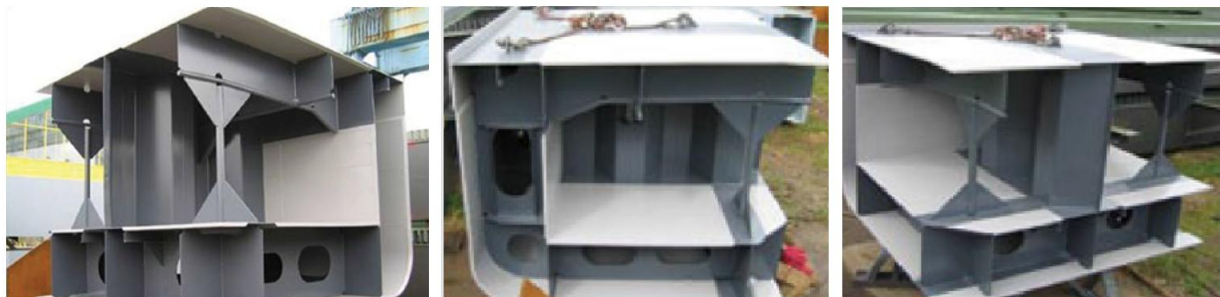
Fig.1.41 The model of a Type C tanker ship with SPS structure (IE, 2016)
