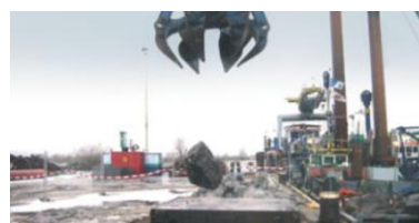
Fig.1.39 Rock impact testing(IE, 2016)
