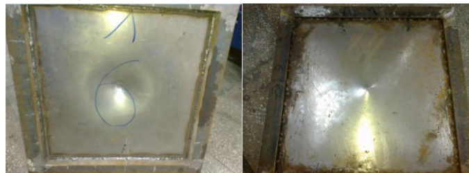
Fig.5.29 – Remanent deformation – model 3
