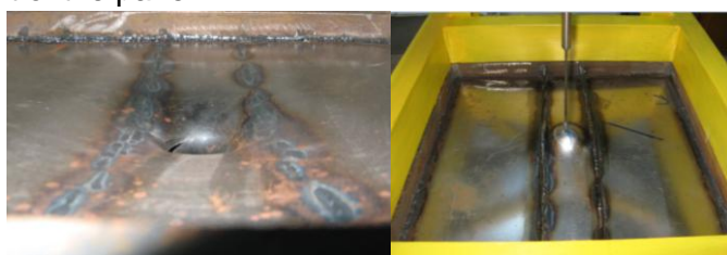
Fig.5.25 – Remanent deformation – model 2
