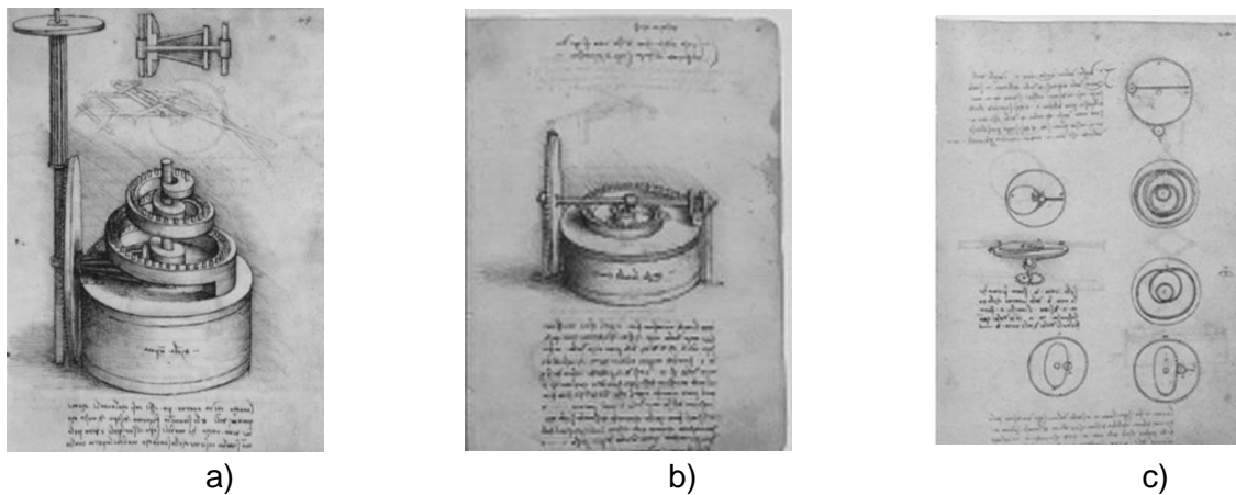
Fig. 1.1. Non-circular gears sketched by Leonardo da Vinci [1]
