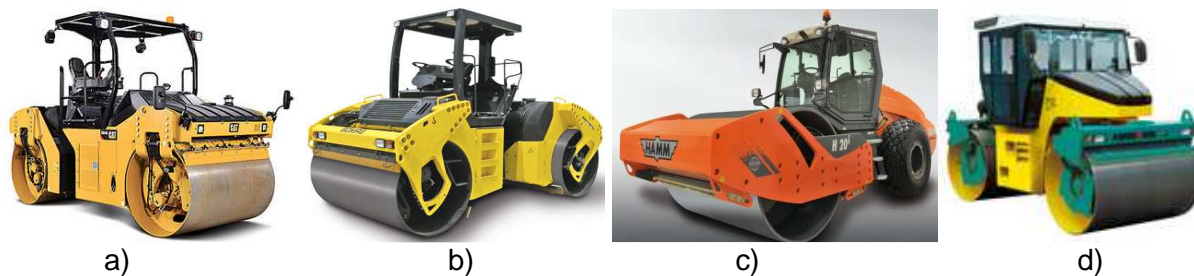
Fig. 2.3 Utilaje de compactare cu două rulouri vibratoare a) model Caterpillar; b) model Bomag; c) model Hamm; d) model Ammann.
