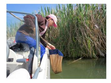
Fig.44 Collecting zoobenthos samples with the limnological net
