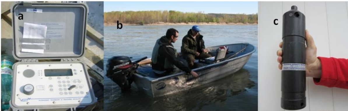
Figure 2 (a) VR100 acoustic receiver, (b) Sturgeon manual / active tracking in Danube River using VR100 acoustic receiver, (c) VR2W acoustic receiver
