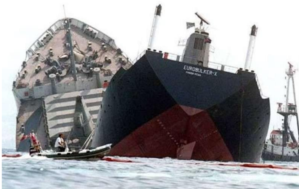
Fig. 1.1.3 – EUROBULKER X Bulk Carrier after breaking, on 02.09.2000, while loading cement at the port of Lefkandi in Greece [8]
