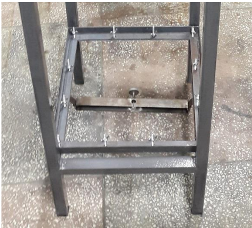
Figura 5.20 Gravitational impact stand. Frame with square support
