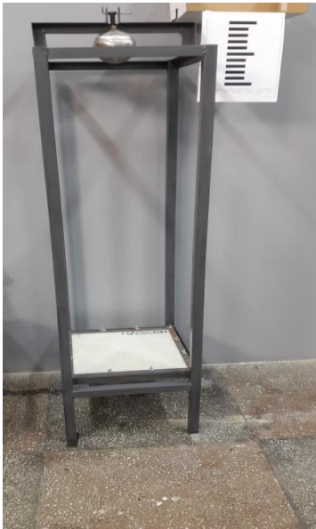
Figure 5.18 Gravitational impact stand with free drop
