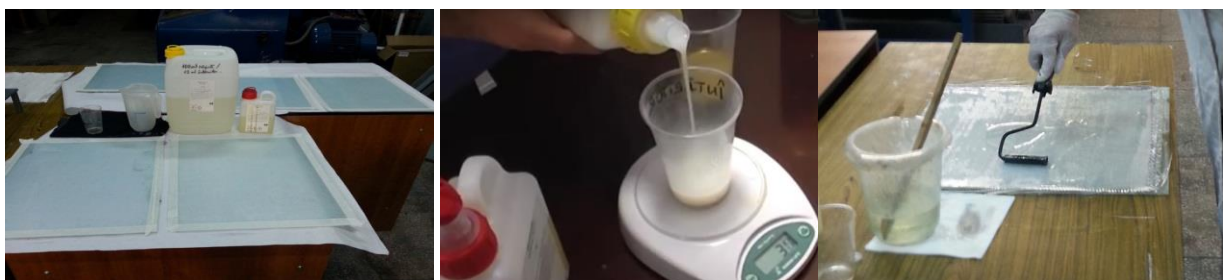
Figure 5.7 Prepare the support glass for casting the epoxy resin a), weighing the solutions and spreading the epoxy resin b), casting c).
