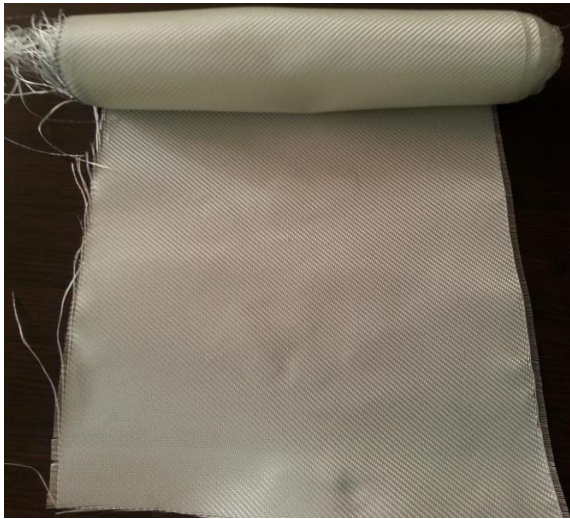
Figure 5.8 Twill texture, 0,2mm thickness
