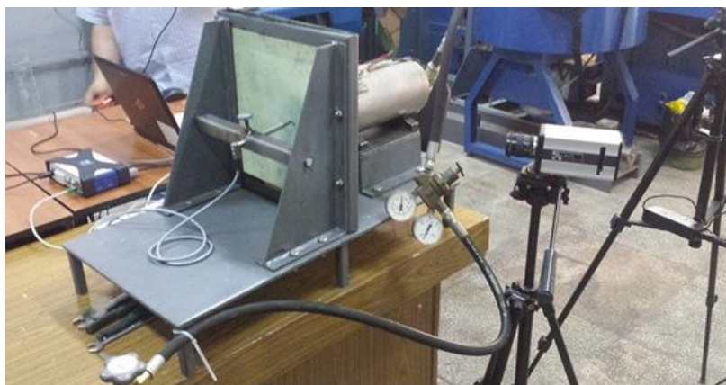
Figure 5.32 Measurement of the plate maximum deformation
