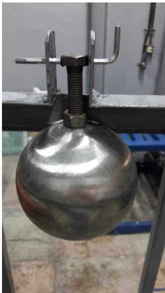
Figure 5.17 Impactor with 5 [kg] mass
