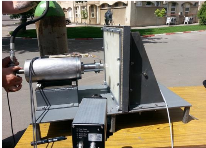
Figure 5.28 Dynamic tests pneumatic stand
