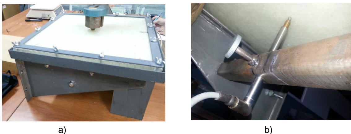
Figure 5.15 a) detail for one of the static tests b) positioning of travelling transducer (LVDT) on the back of sandwich plate
