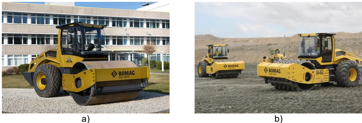
Figure 2.2. Compaction equipment with single degree of freedom for vibratory roller:[1]*** a) smooth vibrating roller; b) profiled vibrating roller (with crampons).
