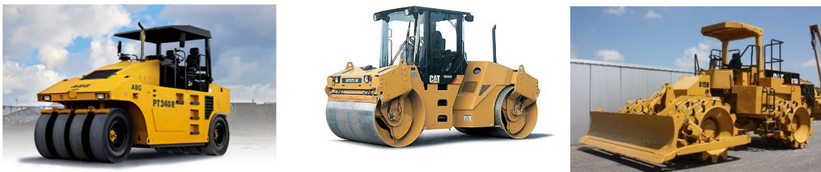
Figure 2.1. Examples of machines that perform static compaction on the ground
