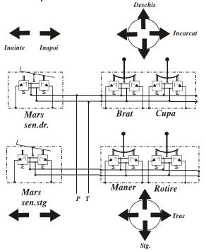
In the case of a tire excavator we have a single hydraulic pump
