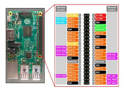
This type of microcomputer has the advantage that each pin can be ordered through the user's written program. The programming language is Pyton a high-level, easy-to-write programming language (uses white spaces for block delineation) that allows for clear instructions.
