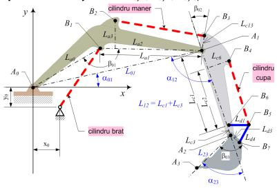
Taking into account the structural and functional geometric parameters, indicate on the model in Figure 4.8 and using the following notations necessary to simplify the final expression formulation
