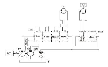
*The LOAD SENSING (LS)* operation of the wheel excavators consists of adjusting the LS of the pump cylinder and using the hydraulic distributors.
