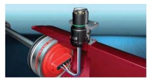
In this case, the cylinder dispenser is also the one that has the role of regulating its movement, both in terms of its travel speed and its stopping at a certain position. For this operation, the board has the ability to change the frequency of the signal so that the distributor plunger can be placed anywhere in the race
