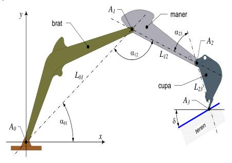
Evaluate the trajectory of the bucket according to its structural parameters ( $L_{01}$ ,  $L_{12}$ ,  $L_{23}$ ) and functional ones (x A3 and y A3), base in the coordinate system xOy, is done in accordance with the schematic of Fig. 4.3. Under these circumstances, the vertical coordinates of the cutting edge of the workpiece (bucket) are given by the following expressions:
