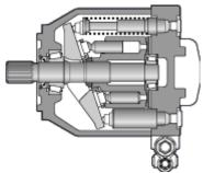
Variable flow pumps having an inclined disk are most suited to using the pressure control with the help of a single microcomputer. For these pumps a hydraulic compensator can also be used on the basis of the pressure differential  $\Delta P$  given by a variable section orifice, this method being most suitable for mechanical adjustment (manual or mechanical devices)
