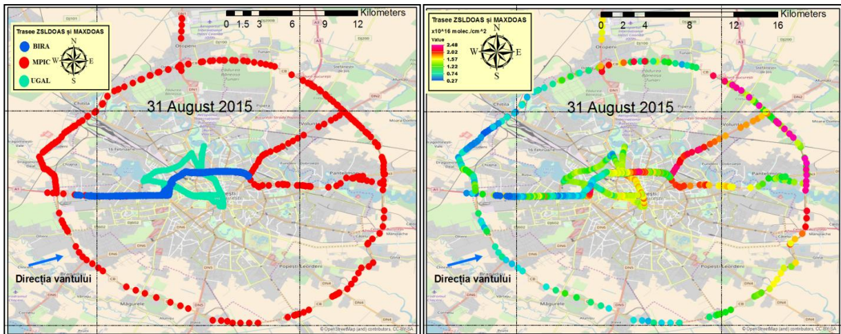
Figura 4.27: Comparison between VCD_{\text{tropo}} \text{NO}_2 detected by the MAX - DOAS MPIC system and the ZSL - DOAS UGAL and BIRA systems on 31.08.2015 in the 09:00: 14:00 UTC (left). Route of the three DOAS systems (right).
