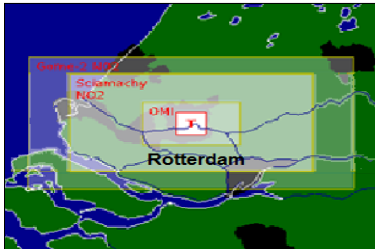
Figure 4.2: Spatial pixel coverage of DOAS satellite instruments used in NO 2 monitoring. Comparison over Rotterdam, The Netherlands. (adapted from http://www.tropomi.eu )
