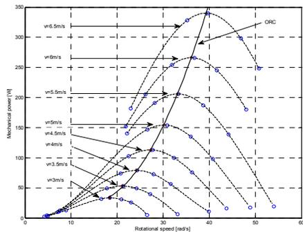
Fig.3. Mechanical power versus wind shaft rotational speed
