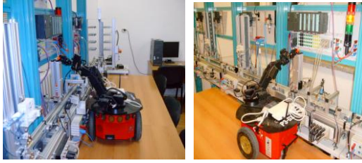
Fig. 1. Assembly line, Hera, served by WMR, Pioneer 3-DX, equipped with RM, Pioneer 5-DOF Arm
