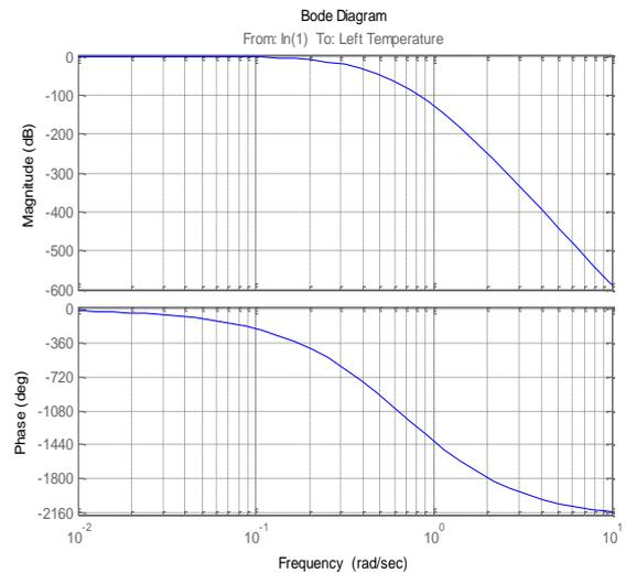
Fig.2. Bode Plot of the full-order system from figure 1, with 25 states in one branch.
