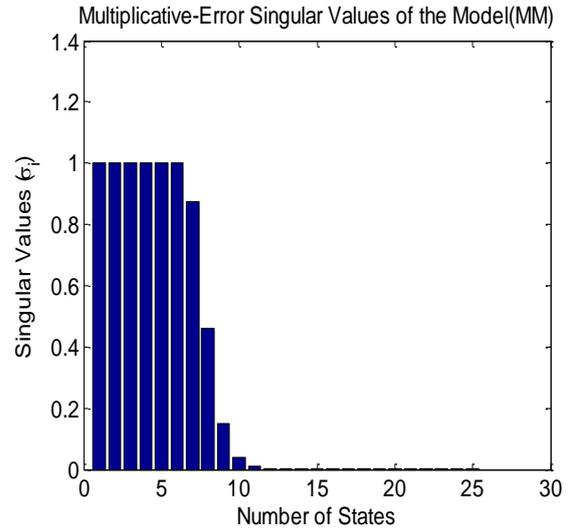
Fig.5. Selection of the 8 dominant states minimally necessary to preserve the dominant dynamics of the original system over one branch of figure 1 computed through the second method (multiplicative error method).
