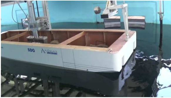
Figure 3.12.a. Experimental SV model, v=0 m/s, T6 , \mu=0^\circ , stern view
