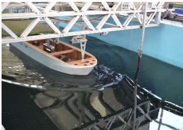
Figure 3.7. The research vessel model at head wave condition
