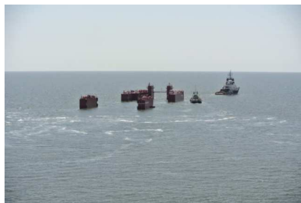
Figure. 1.2. ATLANTE II barge totally submerged in the Black Sea during a launch [11]
