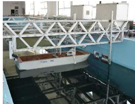
Figure 3.8. The research vessel model at beam wave condition
