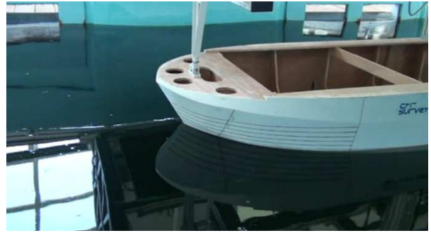
Figure 3.12.b. Experimental SV model, v=0 m/s, T6 , \mu=0^\circ , bow view
