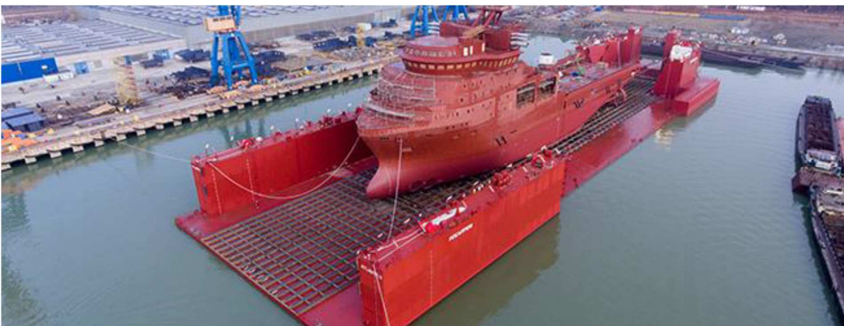
Figure. 1.3. The floating dock Dock_VARD_Tulcea at the end of the total docking of the calculation case in the chapter 7.2.2. [12]
