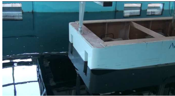
Figure 3.11.b. Experimental SV model, v=0 m/s, T4 , \mu=180^\circ , stern view
