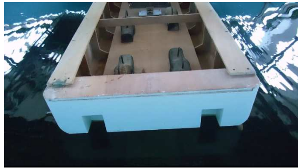
Figure 3.13.b. Experimental SV model, v=0 m/s, T8, \mu=90^\circ , stern view
