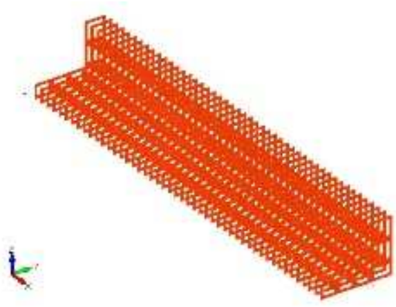
Figure 4.15. Dock60_CWT 3D-CAD/FEM model, longitudinal and frame elements
