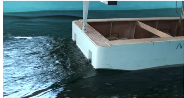
Figure 3.10.b. Experimental SV model, v=1.28 m/s, T4 , \mu=180^\circ , stern view
