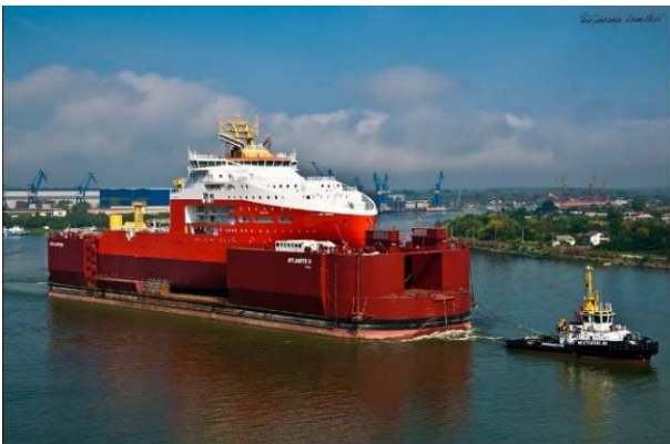
Figure.1.1. ATLANTE II barge on the Danube, having docked a ship that was launched in the Black Sea [10]
