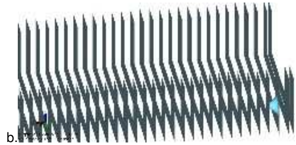
Figure 5.19.a., b. Buckling criteria verification, light case, Dock60_CWT, \mu = 45^\circ , wave height h_w=1.930m a. hogging type wave, b. sagging wave type
