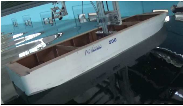
Figure 3.13.a. Experimental SV model, v=0 m/s, T8, \mu=90^\circ , starboard view
