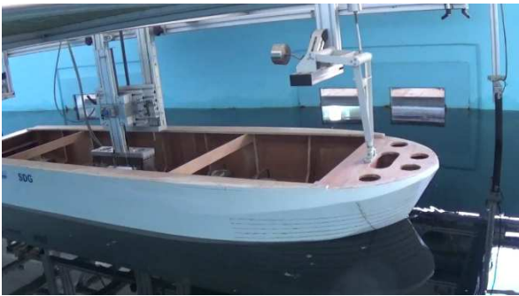
Figure 3.11.a. Experimental SV model, v=0 m/s, T4 , \mu=180^\circ , bow view
