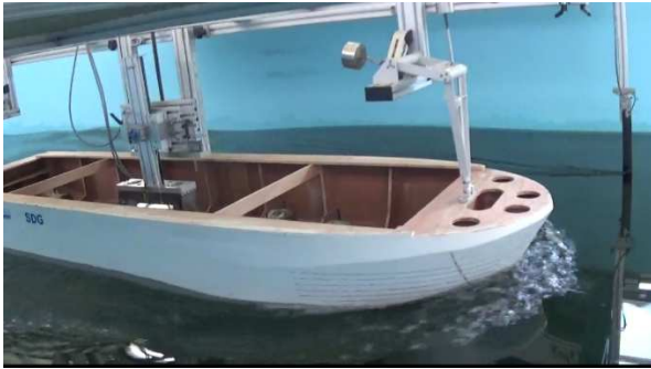
Figure 3.10.a. Experimental SV model, v=1.28 m/s, T4 , \mu=180^\circ , bow view
