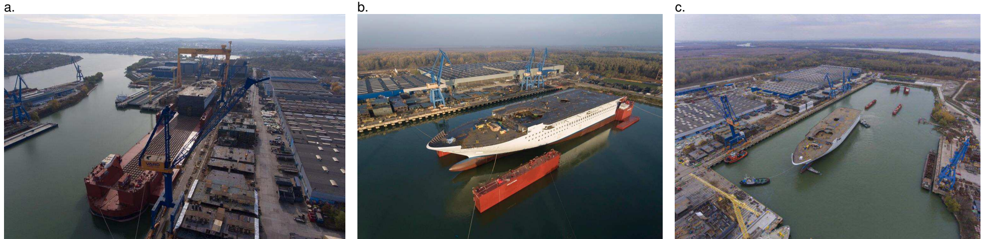
Figure 4.30.a., b., c.. Docking of a ship and launching it into the harbour of the shipyard [74], [75], [76]
