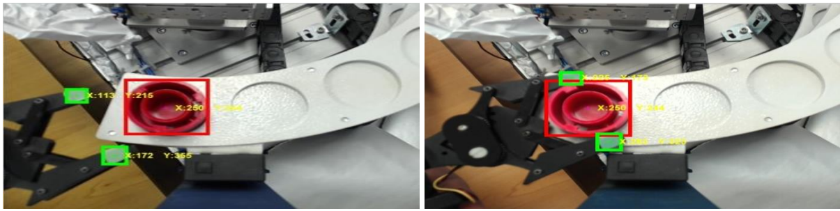
Fig.4.34. Real-time image in which RM Pioneer 5-DOF Arm picks up over the reprocessing piece
