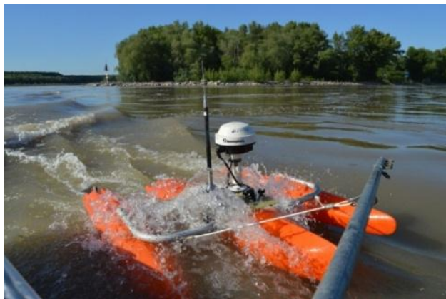
Figure 5.5 Single beam measurement of the riverbed in the location of the monitoring stations
