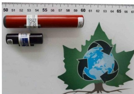
Figure 4.11 Ultrasonic tags (model V13TP-1x and V16TP-6x)
