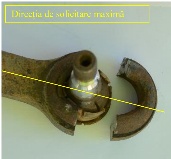
Figure 4. 5 Cross-sectioned tie rod end
