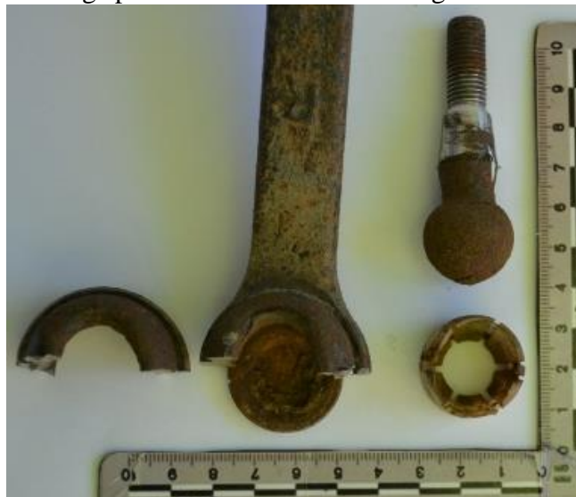
Figure 4. 2 Dacia Logan tie rod end section
