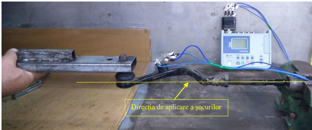
Figure 5. 1 The devices position on the test bench
