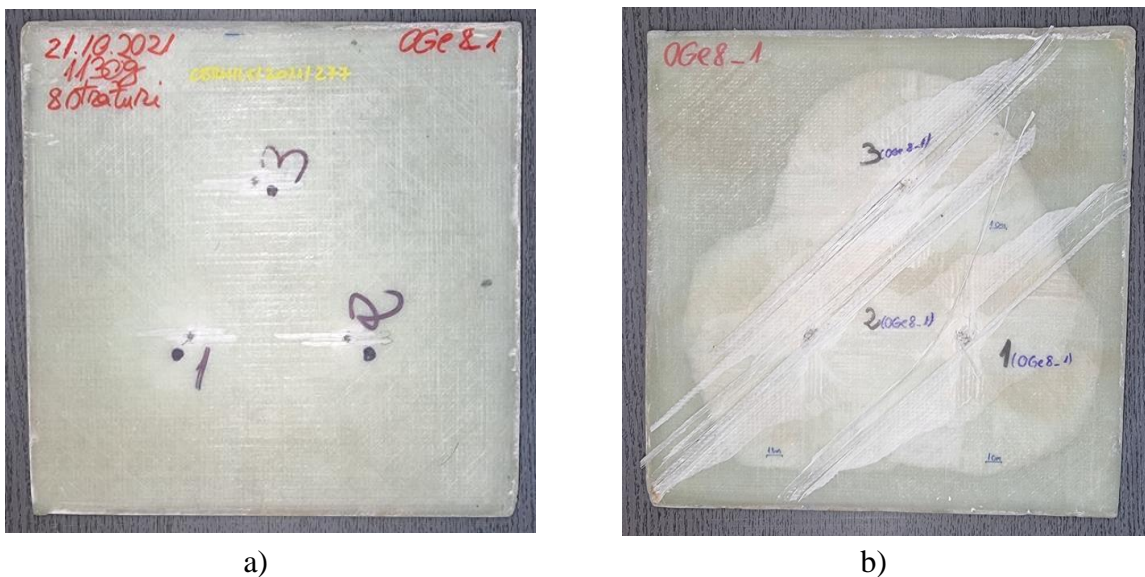
Fig. 5.5. The 8-layer panel after being tested, a) front, b) back
