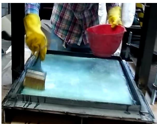
Fig. 4.8. Laying-up process of layers with the mix resin+hardener
