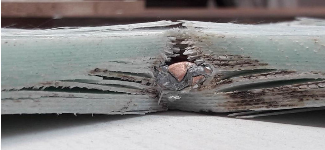
Fig. 1.6. Composite with glassfiber and resin, 13 mm thick, after impact with 9 mm FMJ projectile, at a speed of 420 m/s [22].
