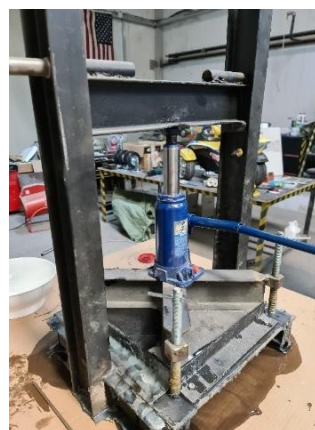
Fig. 4.9. The press for fabricating the panels coded OGe
