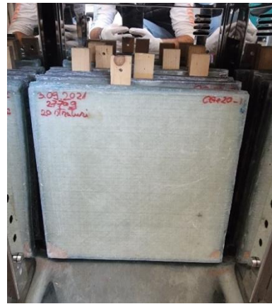
Fig. 4.11. Arrangement of the panels in the oven, with spacers made of wood, for the set of panels with 20 layers
