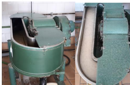
Figure 2.9. Valley beater hollander machine for pulp grinding at laboratory level (source: Căpriță, F.C., Fiber Pulp Preparation Laboratory -Cephart SA Brăila)
