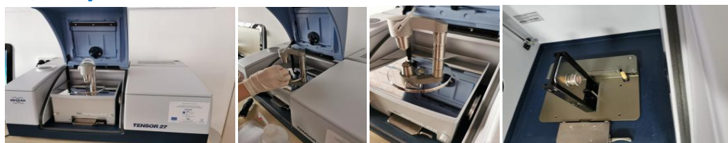
Figure 2.18. Bruker Tensor 27 FTIR spectrometer, coupled with diamond crystal ATR device [Căpriță, F.C., et al., 2022]
