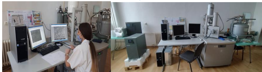
Figure 2.17. Scanning Electron Microscope (SEM) (source: Căpriță, F.C., Electron Microscopy Laboratory, Faculty of Science and Environment - UDJG)
