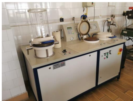
Figure 2.14. Rapid Köthen trainer (source: Căpriță, F.C., Fiber Paste Preparation Laboratory -Cephart SA Brăila)
