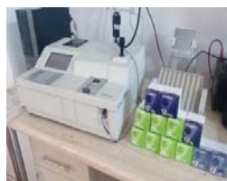
Image 3.6. The VetTest® chemical analyzer and compatible kits for determining serum parameters (original image)
