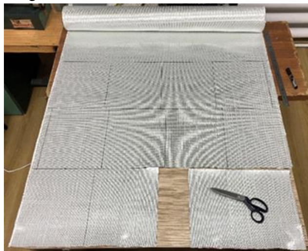
Fig. 4.3. Manufacturing the quadriaxial fabric sheets
