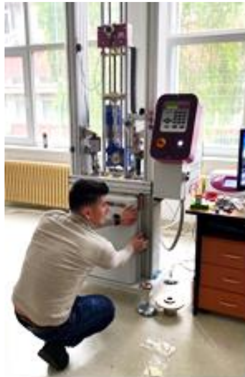
Fig. 4.7. Instron CEAST 9340 low velocity impact testing machine - [57] during testing
