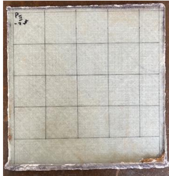
Fig. 4.5. Marking the test samples on the formed composite panels
