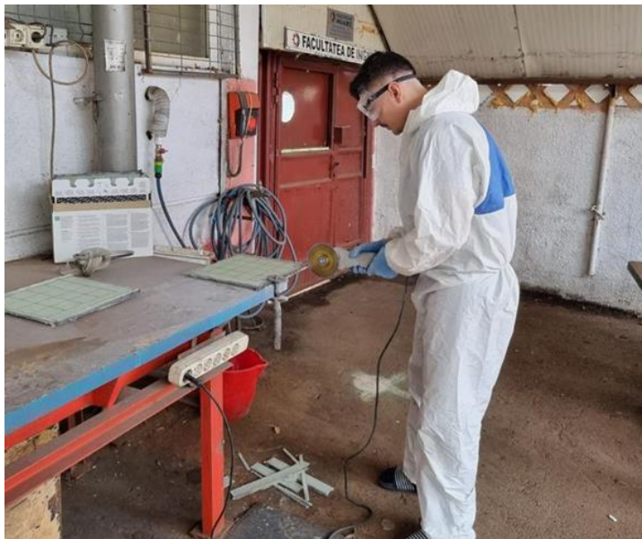
Fig. 4.6. Cutting the samples from the composite panel
