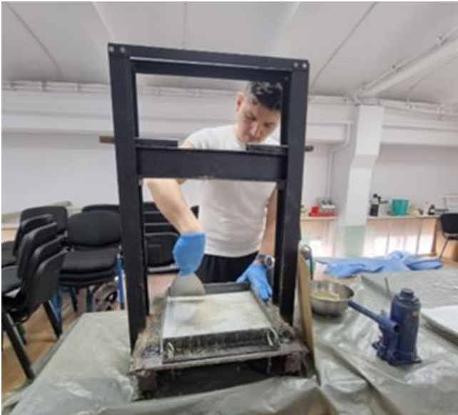
Fig. 4.4. The press in which the sheets were placed
