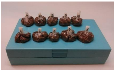
Figure 2.9. Method of packaging of raw samples of waste containing mercury and mercuric salts
