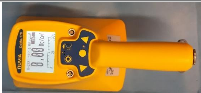
Figure 2.32. Contaminometer CoMo 170 Nuvia Instruments – property of SetCar S.A. Brăila (source: adapted according to [Sloată and Ene, 2021a, b])
