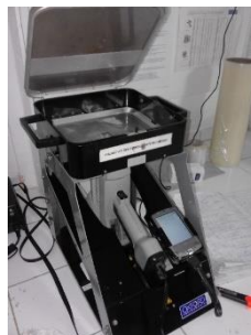
Figure 2.22. ED-XRF spectrometer, X-MET 5000, Oxford Instruments (source: adapted according to [Ene and Sloată, 2017], [Sloată and Ene, 2017a, b])
