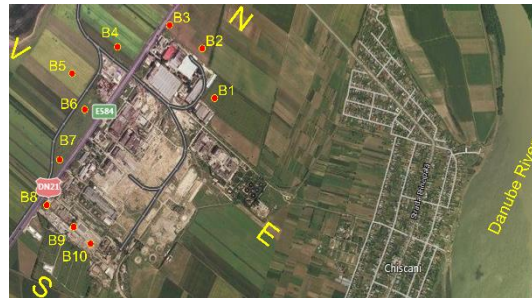
Figure 2.6. Map of soil sampling around the former artificial fiber, pulp and paper plant in Brăila (source: processed according to [Ene and Sloată, 2021], [Ene et al., 2022b], [Sloată et al., 2022a, d])
