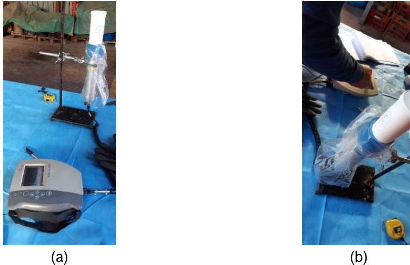
Figure 2.30. Canberra Inspector 1000 portable gamma ray spectrometer – property of RATEN ICN Pitesti: (a) Canberra Inspector 1000 spectrometer and (b) IPROL - 1 probe (source: adapted according to [Sloată and Ene, 2021a, b])
