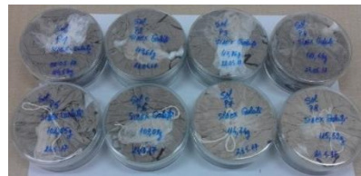
Figure 2.19. Packaging in sarpagan type containers of soil samples taken from around the Liberty Galați metallurgical complex, in order to carry out the GRS analysis
