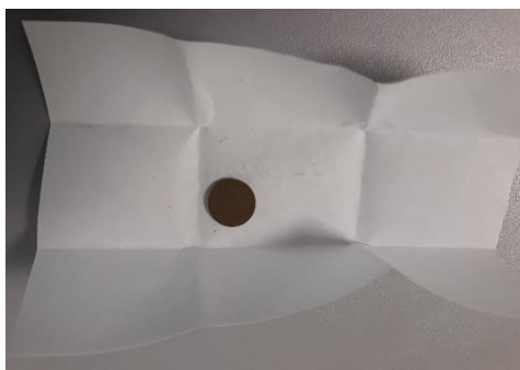
Figure 2.11. Samples prepared for IBA analysis: (a) and (b) samples provisionally packed in paper envelopes, (c) positioning of the samples on the support
