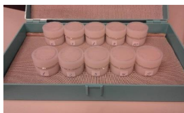
Figure 2.14. Preparation and encapsulation of solid waste samples resulting from pickling processes of metal parts (source: adapted according to [Ene et al., 2021b])
