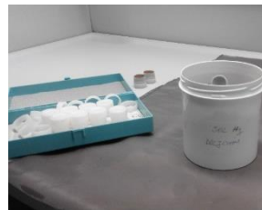
Figure 2.10. Preparation and encapsulation of solid waste samples containing mercury and mercury salts
