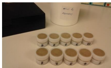
Figure 2.15. Preparation and encapsulation of sand waste samples contaminated with arsenic (source: adapted according to [Ene and Sloată, 2020])
