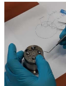
Figure 2.11. Samples prepared for IBA analysis: (a) and (b) samples provisionally packed in paper envelopes, (c) positioning of the samples on the support
