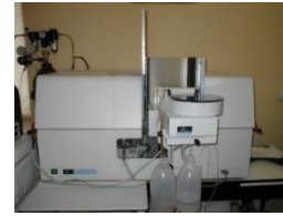
Figure 2.25. AAS AAnalyst800 spectrometer from the IGS laboratory, Chișinău, Republic of Moldova (source: adapted according to [Ene et al., 2019c])
