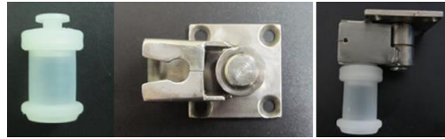
Figure 2.18. The teflon container used for sample packaging and its handling mechanism (source: adapted according to [Pavlov et al., 2016])
