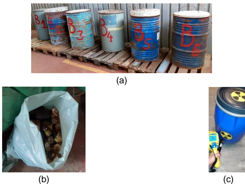
Figure 2.5. Method of packaging of unknown radioactive solid waste (source: adapted according to [Sloată and Ene, 2021b])
