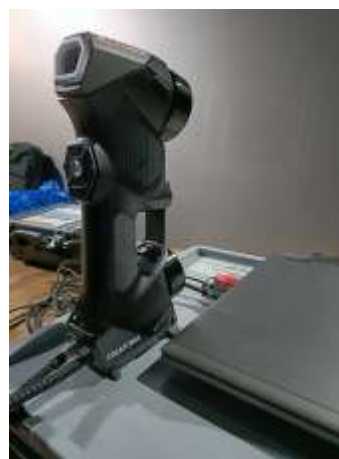
Figura 5.2. Scannerul 3D HANDYSCAN
