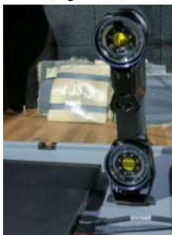
Figura 5.2. Scannerul 3D HANDYSCAN
