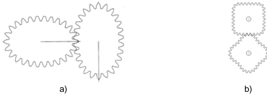
Fig. 1.4. Noncircular gears with continuous variable speed a) elliptical gears [20]; b) four lobes noncircular gears [21]
