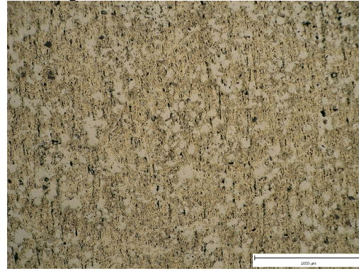
Figure 3.17. Micrograph of composite material A6061/FS45, Stir Casting Vortex method (10 min) and d_{mp} = 0.04 mm (without attack)
