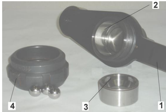
Fig. 3.1. Fixed balls cup. 1 - lever on which the tensiometric mark is mounted, 2 - Fixed balls cup, 3 - ball fastening ring, 4 - ball fastening nut
