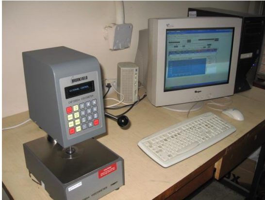
Fig. 5.1. Brookfield Viscosimeter (Department of Machine Design and Tribology, Politehnica University of Bucharest)
