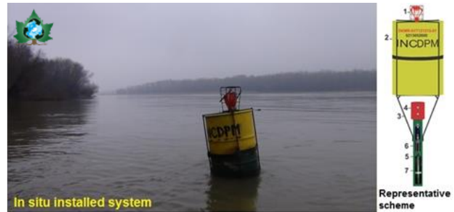
(1) light warning system; (2) floating sheet tank; (3) connecting system between tank and protection pipe; (4) protective cover; (5) protective tube provided with slots; (6) multiparameter used for the quality parameters monitoring; (7) automatic ultrasonic receiver for ichthyofauna monitoring.
