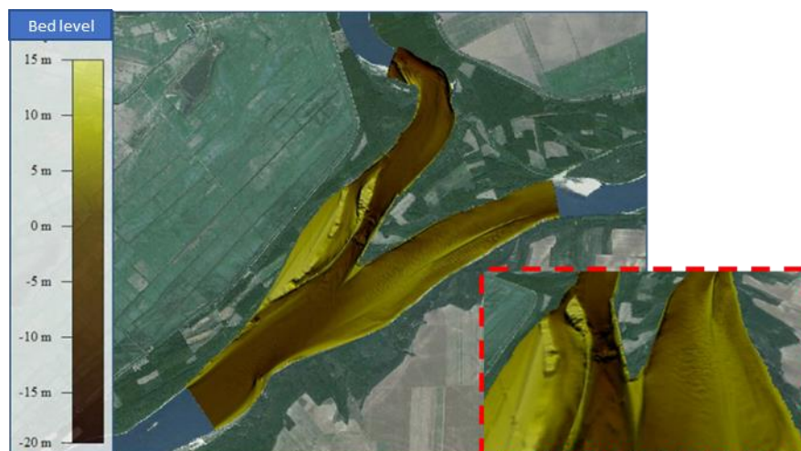
Figure 45 The riverbed relief resulted from the morphohydrodynamic model - calibration step. Bifurcation area detail
