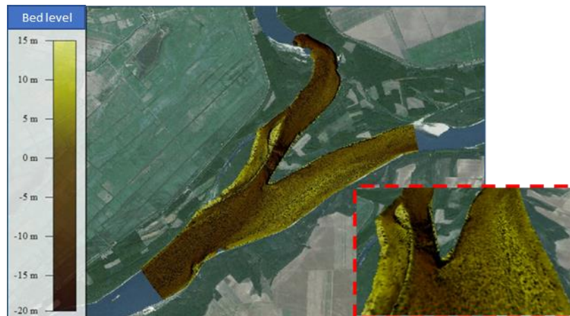
Figure 44 The riverbed relief resulted from bathymetric multibeam measurements performed in the VII year of analysis. Bifurcation area detail
