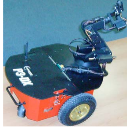
Fig. 1. Pioneer 3-DX with 5-DOF robotic manipulator
