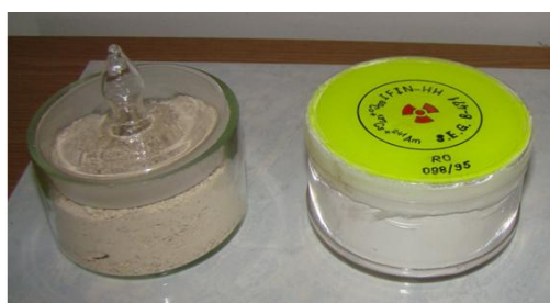
Figure 2.12 - The radioactive source used for calibration of the spectrometer and the measuring sample - identical geometry
