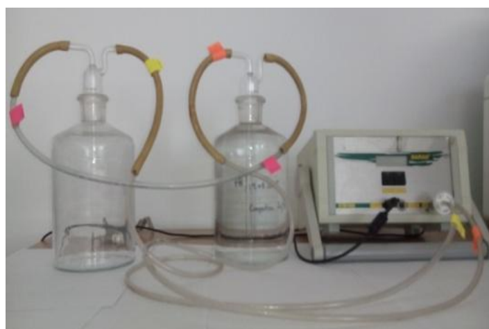
Figure 2.6 - SARAD RTM-1688-2 measuring system for ^{226}\text{Ra}/^{222}\text{Rn} in water [Pintilie V., 2016b]
