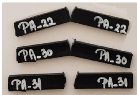
Fig. 6.21. Breaking of specimens following Charpy tests, for material PA6m
