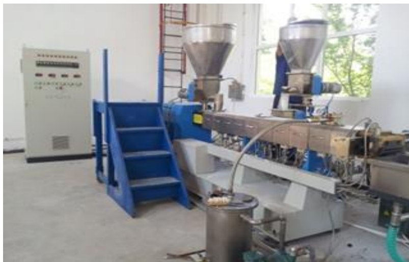
Fig. 3.3. EC 52 double screw granulator extruder (SC Monofil Săvinești SA)
