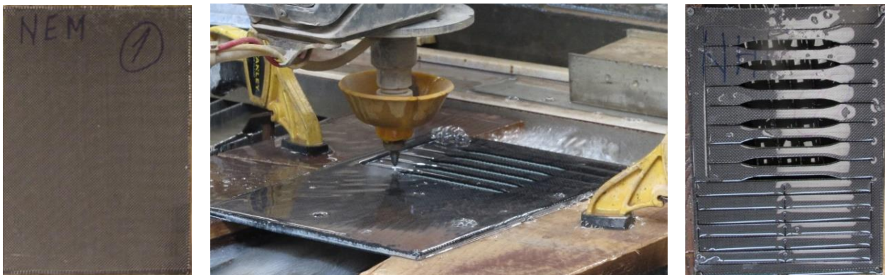
Fig. 5 Steps for extracting the specimens, using the water jet cutting machine (from left to right: pseudo-laminate extracted from the mold; cutting the pseudo-laminate; specimens before extraction from the pseudo-laminate)
