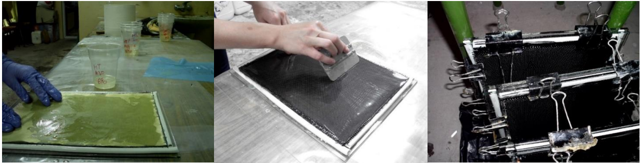
Fig. 4 Formation of pseudo-laminates by hand lay-up method (from left to right: layering; gas evacuation; mold polymerization)
