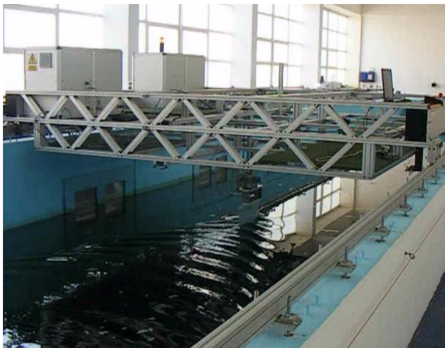
Figure 3.2. Towing tank carriage during tests
